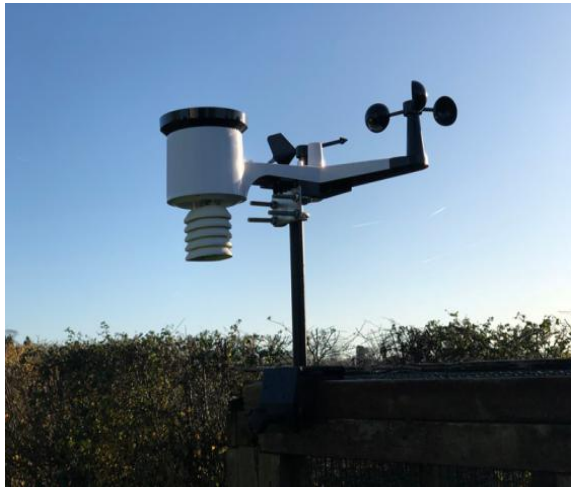
Figure 11.17 - B-Fluid On-site Weather Station
